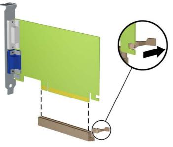
Figure 5-12 Removing a PCI Express x16 Expansion Card
